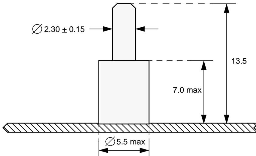
6. The standoff pillars and the CMC bezel front panel are mounted on the S-LINK cards. The keying pins are mounted on the motherboard. To avoid ground loops and antenna effects, the standoff pillars, attachment areas, keying pins, keying holes and CMC bezel front-panel (if fitted) are to be grounded or isolated as described in Table 17 and Table 18.
