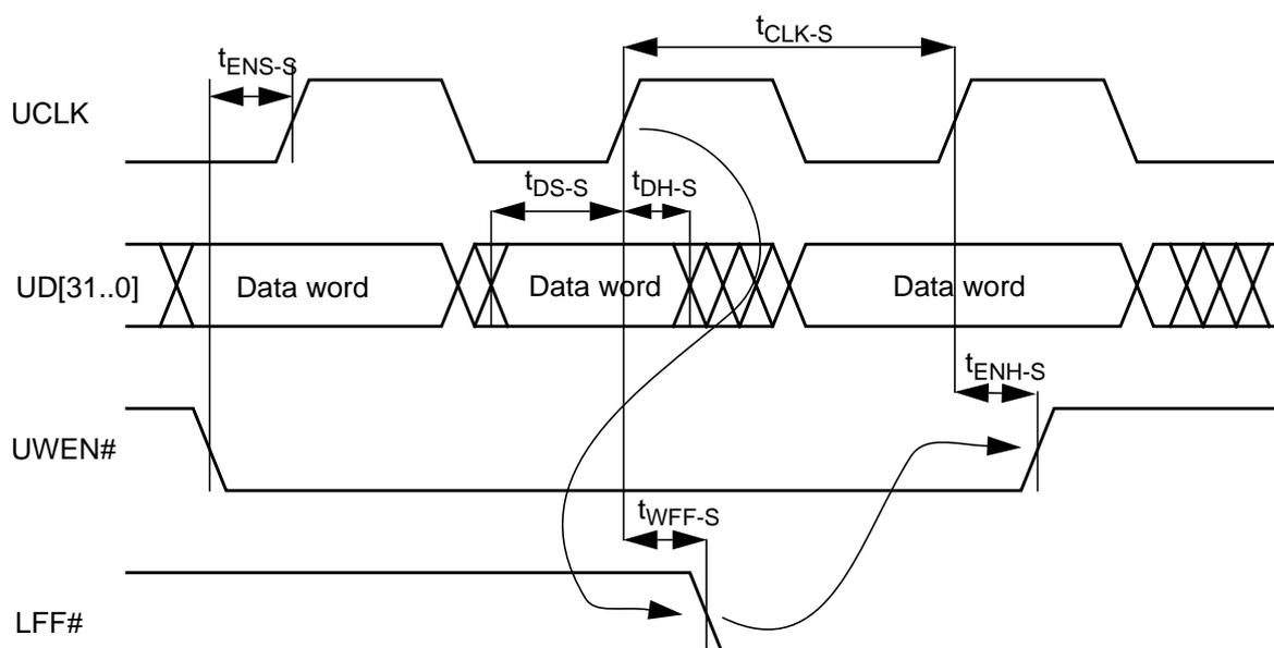
Note: In this diagram, only one extra data word is transferred after LFF# goes low. In fact, up to two words may be transferred.
