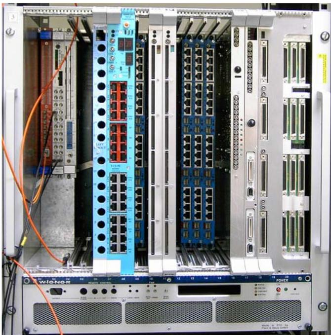
Figure 1 Global Trigger crate with prototype modules
